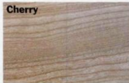
Left: finish wiped on Right: finish brushed on Both have shellac sealer coat
