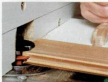
Rout rail ends
