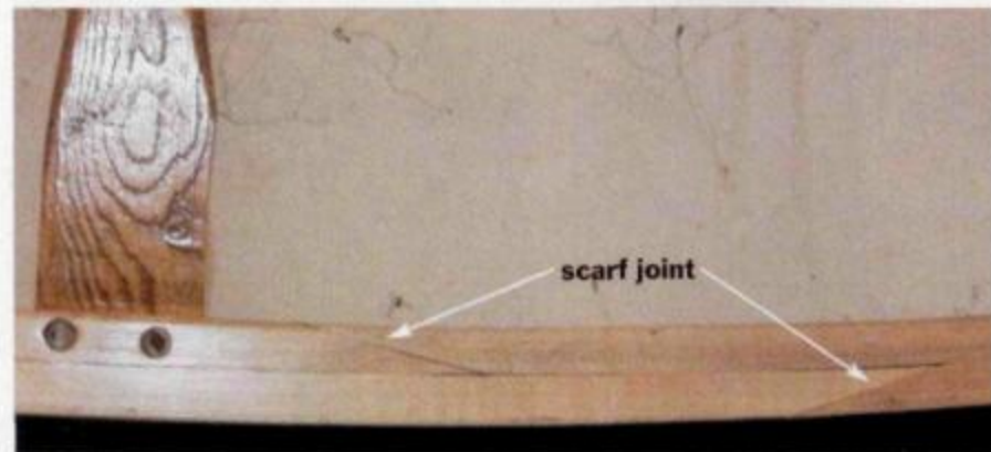
New gunwale showing scarf joint
